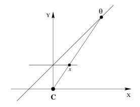
Fig. A3.1. The imaging setup for a simple estimation problem. A point on the line Y = X + 1 is imaged by a line camera. The projection mapping is given by  $f : \theta \mapsto x = \theta/(1+\theta)$ , where  $\theta$  parametrizes the points on the line Y = X + 1. Measurement is subject to noise with a zero-mode distribution.
