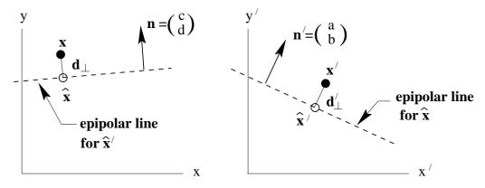
Fig. 14.3. The MLE of  $\mathbf{F}_{A}$  from a set of measured corresponding points  $\{\mathbf{x}_{i} \leftrightarrow \mathbf{x}_{i}'\}$  involves estimating the five parameters a, b, c, d, e together with a set of correspondences  $\{\hat{\mathbf{x}}_{i} \leftrightarrow \hat{\mathbf{x}}_{i}'\}$  which exactly satisfy  $\hat{\mathbf{x}}_{i}'^{\mathsf{T}}\mathbf{F}_{A}\hat{\mathbf{x}}_{i} = 0$ . There is a linear solution to this problem.
