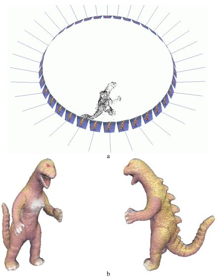
Fig. 19.8. **Dinosaur:** (a) 3D scene points (about 5000) and camera positions for the Dinosaur sequence. (b) The automatic computation of a 3D graphical model for this sequence is described in [Fitzgibbon-98b].
