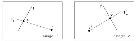
Fig. 13.5. The epipolar geometry induces a homography between corresponding lines  $\mathbf{l} \leftrightarrow \mathbf{l}'$  which are the images of a line  $\mathbf{L}$  in 3-space. The points on  $\mathbf{l}$  are mapped to points on  $\mathbf{l}'$  as  $\mathbf{x}' = [\mathbf{l}']_{\times} F\mathbf{x}$ , where  $\mathbf{x}$  and  $\mathbf{x}'$  are the images of the intersection of  $\mathbf{L}$  with the epipolar plane corresponding to  $\mathbf{l}_e$  and  $\mathbf{l}'_e$ .
