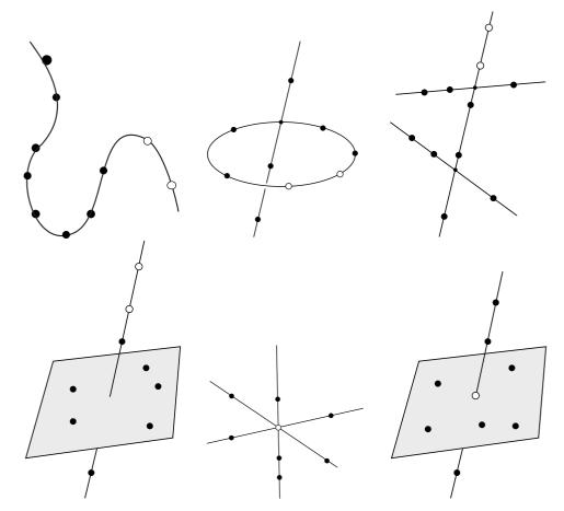
Fig. 22.3. The different critical configurations for camera resectioning from a single view. The open circles represent centres of projection and the filled circles represent points. Each case consists of an algebraic curve (or single point) C containing the camera centres, plus a set of linear subspaces (lines or planes).
