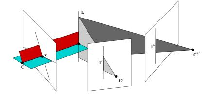
Fig. 17.2. A point–line–line correspondence  $\mathbf{x} \leftrightarrow \mathbf{l}' \leftrightarrow \mathbf{l}''$  involving three images may be interpreted as follows. Two arbitrary lines are chosen to pass through the point  $\mathbf{x}$  in the first image. The four lines then back-project to planes that meet in a point in space.
