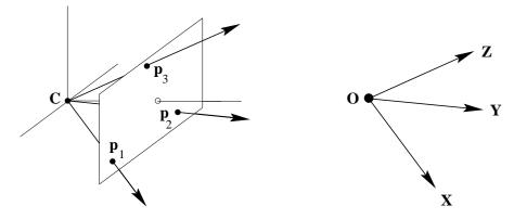
Fig. 6.4. The three image points defined by the columns  $\mathbf{p}_i$ , i = 1, ..., 3, of the projection matrix are the vanishing points of the directions of the world axes.
