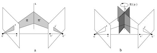
Fig. 13.4. (a) Image lines 1 and 1' determine planes  $\pi$  and  $\pi'$  respectively. The intersection of these planes defines the line L in 3-space. (b) The line L in 3-space is contained in a one parameter family of planes  $\pi(\mu)$ . This family of planes induces a one parameter family of homographies between the images.
