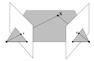
Fig. 10.1. **Triangulation.** The image points  $\mathbf{x}$  and  $\mathbf{x}'$  back project to rays. If the epipolar constraint  $\mathbf{x}'^{\mathsf{T}} \mathbf{F} \mathbf{x} = 0$  is satisfied, then these two rays lie in a plane, and so intersect in a point  $\mathbf{X}$  in 3-space.
