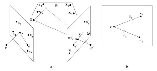
Fig. 13.9. The fundamental matrix is defined uniquely by the image of six 3D points, of which four are coplanar. (a) The parallax for one point **X**. (b) The epipole determined by the intersection of two parallax lines: the line joining  $\tilde{\mathbf{x}}'_5 = H\mathbf{x}_5$  to  $\mathbf{x}'_5$ , and the join of  $\tilde{\mathbf{x}}'_6 = H\mathbf{x}_6$  to  $\mathbf{x}'_6$ .
