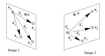
Fig. 14.7. **Reconstruction from two images.** The affine coordinates of the 3D point **X** with image  $\mathbf{x}, \mathbf{x}'$  in two views may be computed linearly from the projection of the basis points  $\mathbf{x}_i$  and basis vectors  $\tilde{\mathbf{e}}_i$  of figure 14.6.
