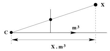
Fig. 6.6. If the camera matrix  $\mathbf{P} = [\mathbf{M} \mid \mathbf{p}_4]$  is normalized so that  $\|\mathbf{m}^3\| = 1$  and det  $\mathbf{M} > 0$ , and  $\mathbf{x} = w(x, y, 1)^{\mathsf{T}} = \mathbf{P}\mathbf{X}$ , where  $\mathbf{X} = (\mathbf{X}, \mathbf{Y}, \mathbf{Z}, 1)^{\mathsf{T}}$ , then w is the depth of the point  $\mathbf{X}$  from the camera centre in the direction of the principal ray of the camera.
