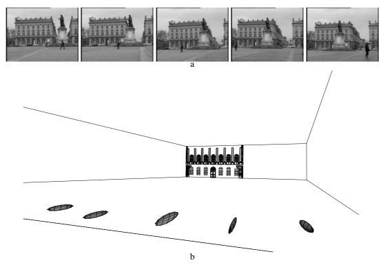
Fig. 7.3. **Camera centre covariance ellipsoids**. (a) Five images of Stanislas square (Nancy, France), for which 3D calibration points are known. (b) Camera centre covariance ellipsoids corresponding to each image, computed for cameras estimated from the imaged calibration points. Note, the typical cigar shape of the ellipsoid aligned towards the scene data. Figure courtesy of Vincent Lepetit, Marie-Odile Berger and Gilles Simon.
