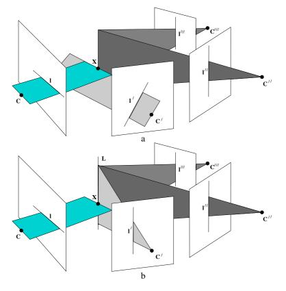
Fig. 17.1. Four line "correspondence". The four lines  $\mathbf{l}, \mathbf{l}', \mathbf{l}''$  satisfy the quadrilinear relation (17.22) since their back-projections intersect in a common point  $\mathbf{X}$ . (a) No three planes intersect in a common line. (b) The three lines  $\mathbf{l}' \leftrightarrow \mathbf{l}'' \leftrightarrow \mathbf{l}'''$  are the image of the same line  $\mathbf{L}$  in 3-space.
