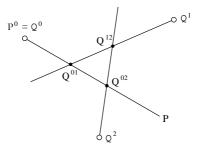
Fig. 22.7. Configuration of the three camera centres and the three ambiguous points. If the three points  $\mathbf{Q}^{ij}$  are distinct, then they all lie in the plane of the camera centres  $\mathbf{C}_{\mathbf{0}}^{i}$ .
