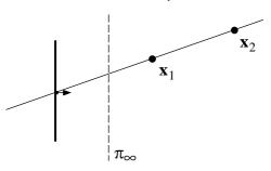
Fig. 21.4. As shown, the point  $\mathbf{x}_1$  is closer to the camera than  $\mathbf{x}_2$ . However, if an orientation-reversing projectivity is applied, taking  $\pi_\infty$  to infinity, then both  $\mathbf{x}_1$  and  $\mathbf{x}_2$  remain in front of the camera, but  $\mathbf{x}_2$  is closer to the camera than  $\mathbf{x}_1$ .
