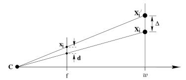
Fig. 7.2. The DLT algorithm minimizes the sum of squares of geometric distance  $\Delta$  between the point  $\mathbf{X}_i$  and the point  $\mathbf{X}'_i$  mapping exactly onto  $\mathbf{x}_i$  and lying in the plane through  $\mathbf{X}_i$  parallel to the principal plane of the camera. A short calculation shows that  $wd = f\Delta$ .
