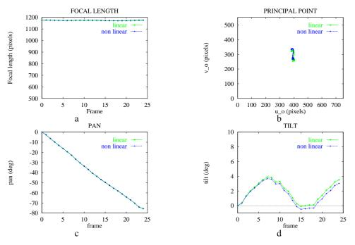
Fig. 19.4. Rotation for varying internal parameters assuming square pixels. These are for the panned sequence of figure 8.9(p206). (a) Focal length. (b) Principal point. (c) Pan angle. (d) Tilt angle. Figures courtesy of Lourdes de Agapito Vicente.
