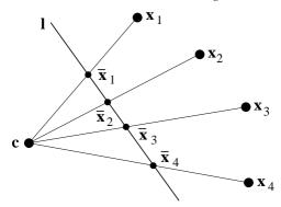
Fig. 22.1. Projection of points in the plane using a 2D camera. A 1D image is formed by the intersection of the rays  $l_i = \overline{cx_i}$  with the image line l. The set of image points  $\{\bar{x}_i\}$  is projectively equivalent to the set of rays  $\{l_i\}$ . For four points, the projective equivalence class of the image is determined by the cross ratio of the points.
