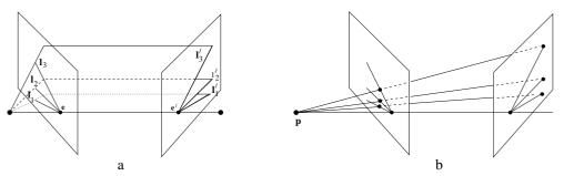
Fig. 9.6. **Epipolar line homography.** (a) There is a pencil of epipolar lines in each image centred on the epipole. The correspondence between epipolar lines,  $l_i \leftrightarrow l'_i$ , is defined by the pencil of planes with axis the baseline. (b) The corresponding lines are related by a perspectivity with centre any point **p** on the baseline. It follows that the correspondence between epipolar lines in the pencils is a 1D homography.
