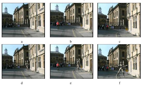
Fig. 1.7. **Augmented video.** The animated robot is inserted into the scene and rendered using the computed cameras of figure 1.3. (a)-(c) Original frames from the sequence. (d)-(f) The augmented frames. Figures courtesy of 2d3 (www.2d3.com).
