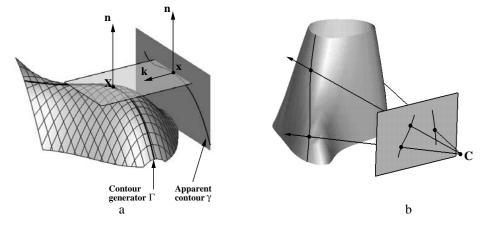
Fig. 8.3. Contour generator and apparent contour. (a) for parallel projection; (b) for central projection. The ray from the camera centre through x is tangent to the surface at X. The set of such tangent points X defines the contour generator, and their image defines the apparent contour. In general the contour generator is a space curve. Figure courtesy of Roberto Cipolla and Peter Giblin.
