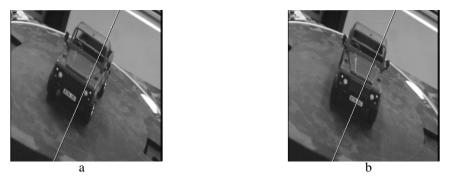
Fig. 14.14. Computing motion from affine epipolar geometry. (a)(b) Two views of a buggy rotating on a turntable. The computed rotation axis is superimposed on the image, drawn to pass through the image centre. The ground truth axis is, of course, perpendicular to the turntable in the world.
