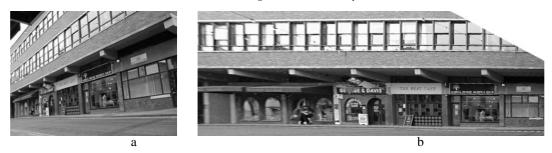
Fig. 8.25. Plane rectification via partial internal parameters (a) Original image. (b) Rectification assuming the camera has square pixels and principal point at the centre of the image. The focal length is computed from the single orthogonal vanishing point pair. The aspect ratio of a window in the rectified image differs from the ground truth value by 3.7%. Note that the two parallel planes, the upper building facade and the lower shopfront, are both mapped to fronto-parallel planes.
