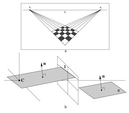
Fig. 8.16. Vanishing line formation. (a) The two sets of parallel lines on the scene plane converge to the vanishing points  $\mathbf{v}_1$  and  $\mathbf{v}_2$  in the image. The line 1 through  $\mathbf{v}_1$  and  $\mathbf{v}_2$  is the vanishing line of the plane. (b) The vanishing line 1 of a plane  $\pi$  is obtained by intersecting the image plane with a plane through the camera centre **C** and parallel to  $\pi$ .
