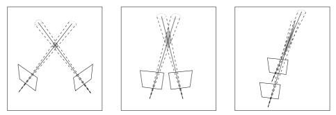
Fig. 12.6. Uncertainty of reconstruction. The shaded region in each case illustrates the shape of the uncertainty region, which depends on the angle between the rays. Points are less precisely localized along the ray as the rays become more parallel. Forward motion in particular can give poor reconstructions since rays are almost parallel for much of the field of view.
