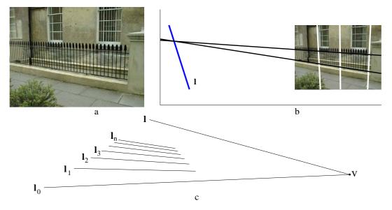
Fig. 8.18. Determining a planes vanishing line from imaged equally spaced parallel lines. (a) Image of a vertical fence with equally spaced bars. (b) The computed vanishing line 1 from three equally spaced bars (12 apart). Note the vanishing point of the horizontal lines lies on this vanishing line. (c) The spacing between the imaged lines  $l_n$  monotonically decreases with n.
