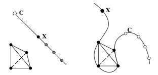
Fig. 22.5. Left: Any point on the line passing through C and X is projected to the same point from projection centre C. Right: The dual statement – from any centre of projection C lying on a twisted cubic passing through X and the vertices of the reference tetrahedron, the five points are projected in the same way (up to projective equivalence). Thus a camera is constrained to lie on a twisted cubic by its image of five known points.
