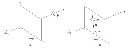
Fig. 14.10. The rotation representation. (a) rotation by  $\theta$  about the Z-axis; (b) subsequent rotation by  $\rho$  about a fronto-parallel axis  $\Phi$  angled at  $\phi$  to the X-axis. The  $\Phi$ -axis has components  $(\cos \phi, \sin \phi, 0)^{\mathsf{T}}$ .
