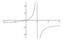
Fig. A3.2. The ML estimate of the world-point position  $\hat{\theta}(x) = f^{-1}(x) = x/(1-x)$  for different measurements of the image point x. Note that for values of x greater than 1, the ML estimate switches to "behind" the camera.
