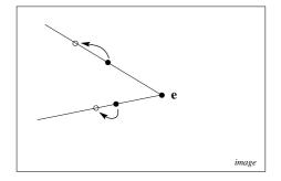
Fig. 11.5. For a pure translation the epipole can be estimated from the image motion of two points.
