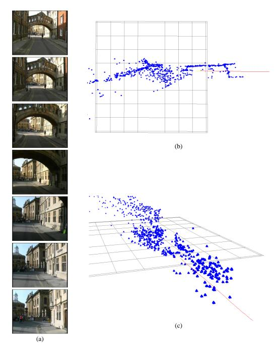
Fig. 1.3. **Reconstruction.** (a) Seven frames of a 700 frame sequence acquired by a hand held camera whilst walking down a street in Oxford. (b)(c) Two views of the reconstructed point cloud and camera path (the red curve). Figures courtesy of David Capel and 2d3 (www.2d3.com).
