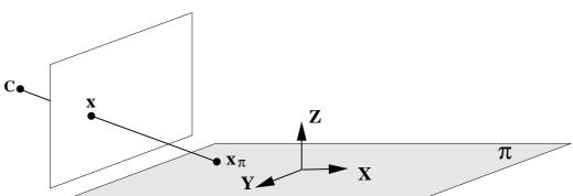
Fig. 8.1. **Perspective image of points on a plane.** The XY-plane of the world coordinate frame is aligned with the plane  $\pi$ . Points on the image and scene planes are related by a plane projective transformation.
