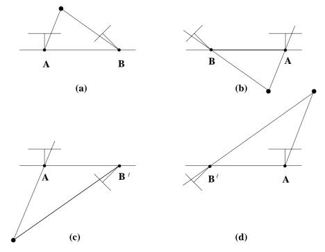
Fig. 9.12. The four possible solutions for calibrated reconstruction from E. Between the left and right sides there is a baseline reversal. Between the top and bottom rows camera B rotates 180° about the baseline. Note, only in (a) is the reconstructed point in front of both cameras.
