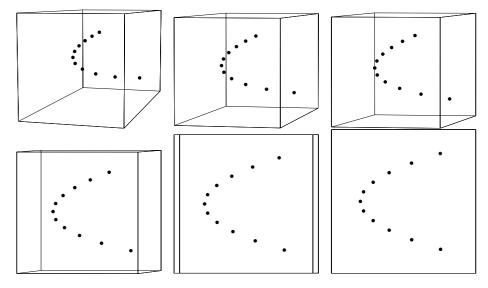
Fig. 22.4. Separate views of a set of points on the twisted cubic  $(t^3, t^2, t, 1)^T$  as viewed from a centre of projection. The visible points are viewed from the points with t = 3, 4, 5, 10, 50, 1000 with the image suitably magnified to prevent the point set from becoming too small. As is plausible from the image, the sets of points differ by a projective transformation. From a viewpoint on a twisted cubic, the twisted cubic has the appearance of a conic, in this particular case a parabola.
