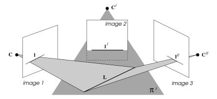
Fig. 15.3. Line transfer. The action on lines of the homography defined by figure 15.2 may similarly be visualized geometrically. A line, l, in the first image defines a plane in 3-space, which intersects  $\pi'$  in the line L. This line L is then imaged as the line l' in the third view.
