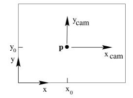
Fig. 6.2. Image (x, y) and camera  $(x_{cam}, y_{cam})$  coordinate systems.
