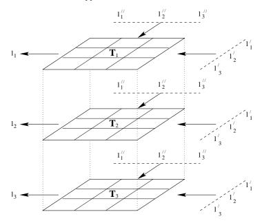
Fig. A1.1. A 3-dimensional representation of the trifocal tensor – figure after Faugeras and Papadopoulo [Faugeras-97]. The picture represents  $l_i = l'_j l''_k \mathcal{T}_i^{jk}$ , which is the contraction of the tensor with the lines l' and l'' to produce a line l. In pseudo-matrix notation this can be written as  $l_i = l'^T T_i l''^T$ , where  $(T_i)_{jk} = \mathcal{T}_i^{jk}$ .
