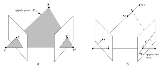
Fig. 9.1. **Point correspondence geometry.** (a) The two cameras are indicated by their centres C and C' and image planes. The camera centres, 3-space point X, and its images x and x' lie in a common plane  $\pi$ . (b) An image point x back-projects to a ray in 3-space defined by the first camera centre, C, and x. This ray is imaged as a line I' in the second view. The 3-space point X which projects to x must lie on this ray, so the image of X in the second view must lie on I'.
