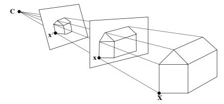
Fig. 8.5. The cone of rays with vertex the camera centre. An image is obtained by intersecting this cone with a plane. A ray between a 3-space point  $\mathbf{X}$  and the camera centre  $\mathbf{C}$  pierces the planes in the image points  $\mathbf{x}$  and  $\mathbf{x}'$ . All such image points are related by a planar homography,  $\mathbf{x}' = \mathbf{H}\mathbf{x}$ .
