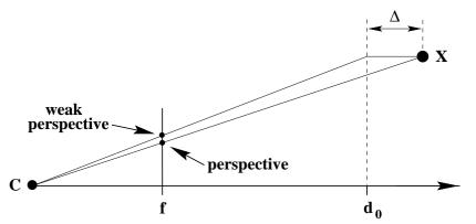
Fig. 6.8. **Perspective vs weak perspective projection.** The action of the weak perspective camera is equivalent to orthographic projection onto a plane (at  $Z = d_0$ ), followed by perspective projection from the plane. The difference between the perspective and weak perspective image point depends both on the distance  $\Delta$  of the point **X** from the plane, and the distance of the point from the principal ray.
