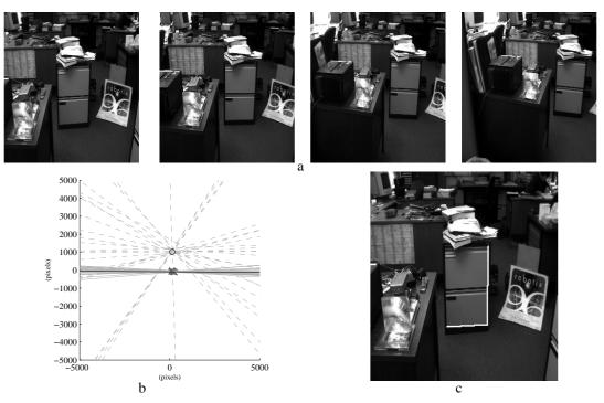
Fig. 19.6. **Planar motion sequence.** (a) Four images (of seven used) acquired from a camera mounted on a vehicle moving on a plane. (b) The computed epipoles  $(\times)$ , horizon lines (grey solid), and imaged screw axes (grey dashed) for all image pairs. (c) Euclidean invariants measured in the metric reconstruction the right angle is measured as  $89^\circ$ , the ratio of the non-parallel lengths is measured as 0.61 (compared to the approximate veridical value of 0.65).
