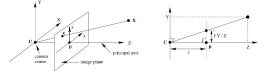
Fig. 6.1. **Pinhole camera geometry.** C *is the camera centre and*  $\mathbf{p}$  *the principal point. The camera centre is here placed at the coordinate origin. Note the image plane is placed in front of the camera centre.*
