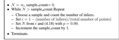
Algorithm 4.5. Adaptive algorithm for determining the number of RANSAC samples.
