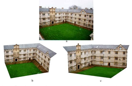
Fig. 8.26. **Single view reconstruction.** (*a*) Original image of the Fellows quad, Merton College, Oxford. (*b*) (*c*) Views of the 3D model created from the single image. The vanishing line of the roof planes is computed from the repetition of the texture pattern.
