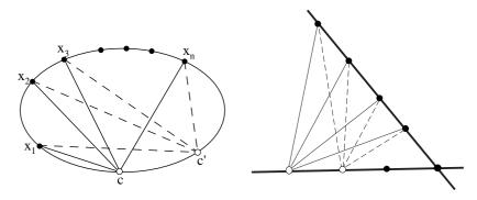
Fig. 22.2. The points  $\mathbf{x}_1, \ldots, \mathbf{x}_n$  project in equivalent ways to the two camera centres  $\mathbf{c}$  and  $\mathbf{c}'$ .
