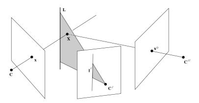
Fig. 15.5. Non-incident configuration. The imaged points and lines of this configuration satisfy the point–line–point incidence relation of table 15.1. However, the space point  $\mathbf{X}$  and line  $\mathbf{L}$  are not incident. Compare with figure 15.4.
