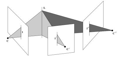
Fig. 15.1. A line L in 3-space is imaged as the corresponding triplet  $\mathbf{l} \leftrightarrow \mathbf{l}' \leftrightarrow \mathbf{l}''$  in three views indicated by their centres,  $\mathbf{C}, \mathbf{C}', \mathbf{C}''$ , and image planes. Conversely, corresponding lines back-projected from the first, second and third images all intersect in a single 3D line in space.
