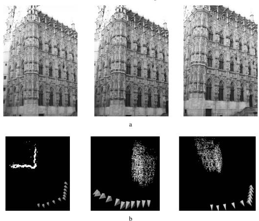
Fig. 1.5. (a) Three high resolution images  $(3000 \times 2000 \text{ pixels})$  from a set of eleven of the cityhall in Leuven, Belgium. (b) Three views of a Euclidean reconstruction computed from the image set showing the 11 camera positions and point cloud.
