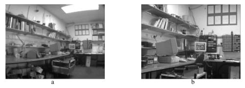
Fig. 7.4. (a) Short vs (b) long focal lengths. Note the curved imaged lines at the periphery in (a) which are images of straight scene lines.
