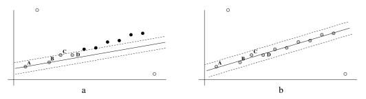
Fig. 4.8. **Robust ML estimation.** The grey points are classified as inliers to the line. (a) A line defined by points  $\langle \mathbf{A}, \mathbf{B} \rangle$  has a support of four (from points  $\{\mathbf{A}, \mathbf{B}, \mathbf{C}, \mathbf{D}\}$ ). (b) The ML line fit (orthogonal least-squares) to the four points. This is a much improved fit over that defined by  $\langle \mathbf{A}, \mathbf{B} \rangle$ . 10 points are classified as inliers.
