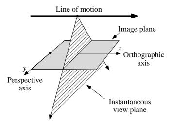
Fig. 6.9. Acquisition geometry of a pushbroom camera.
