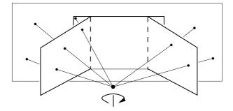
Fig. 8.8. *Three images acquired by a rotating camera may be registered to the frame of the middle one, as shown, by projectively warping the outer images to align with the middle one.*
