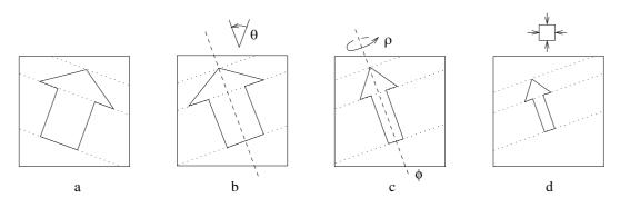
Fig. 14.13. The effect of scale and rotation angles on the epipolar lines for an object moving relative to a stationary camera. This also illustrates the assumed sequence of events accounting for the transition from  $I_1$  to  $I_2$ : (a)  $I_1$ ; (b) cyclotorsion ( $\theta$ ); (c) rotation out of the plane ( $\phi$  and  $\rho$ ); (d) scaling, giving  $I_2$ .
