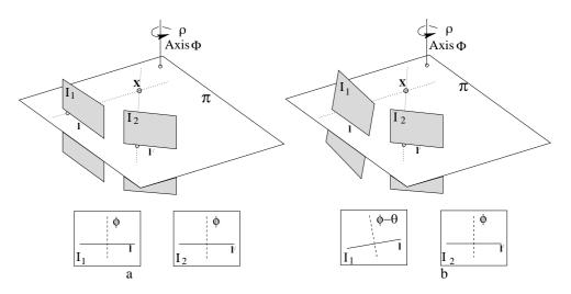
Fig. 14.11. The camera rotates about the axis  $\Phi$  which is parallel to the image plane. The intersection of the epipolar plane  $\pi$  with the image planes gives epipolar lines 1 and 1', and the projections of  $\Phi$  in the images are orthogonal to these epipolar lines: (a) no cyclotorsion occurs ( $\theta = 0^{\circ}$ ); (b) the camera counter-rotates by  $\theta$  in  $I_1$ , so the orientation of the epipolar lines changes by  $\theta$ .
