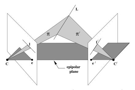
Fig. 12.8. Line reconstruction. The image lines  $\mathbf{l}, \mathbf{l}'$  back-project to planes  $\pi, \pi'$  respectively. The plane intersection determines the line  $\mathbf{L}$  in 3-space. If the line in 3-space lies on an epipolar plane then its position in 3-space cannot be determined from its images. In this case the epipoles lie on the image lines.
