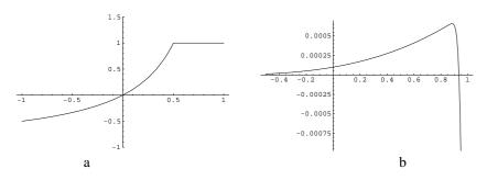
Fig. A3.4. (a) If the range of possible values of the world-point parameter  $\theta$  is limited to the range  $\theta \leq 1$ , then the ML estimate of any point x > 1/2 will be  $\theta = 1$ . This will prevent infinite bias in the estimate, but there will still be bias. (b) The bias  $E_{\theta}[\hat{\theta}(x)] - \theta = \int_{x} \hat{\theta}(x)p(x|\theta)dx - \theta$  as a function of  $\theta$ . Measurement noise is Gaussian with  $\sigma = 0.01$ .
