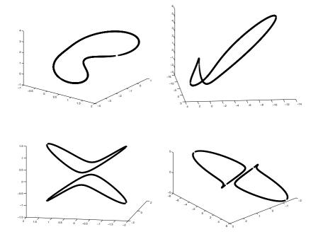
Fig. 22.8. Examples of elliptic quartic curves generated as the intersection of two ruled quadrics.
