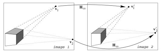
Fig. 13.12. The infinite homography  $H_{\infty}$  maps vanishing points between the images.
