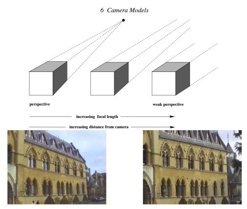
Fig. 6.7. As the focal length increases and the distance between the camera and object also increases, the image remains the same size but perspective effects diminish.
