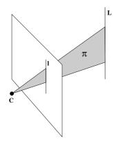
Fig. 8.2. Line projection. A line L in 3-space is imaged as a line 1 by a perspective camera. The image line 1 is the intersection of the plane  $\pi$ , defined by L and the camera centre C, with the image plane. Conversely an image line 1 back-projects to a plane  $\pi$  in 3-space. The plane is the "pull-back" of the line.
