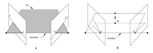
Fig. 9.2. Epipolar geometry. (a) The camera baseline intersects each image plane at the epipoles e and e'. Any plane  $\pi$  containing the baseline is an epipolar plane, and intersects the image planes in corresponding epipolar lines 1 and 1'. (b) As the position of the 3D point X varies, the epipolar planes "rotate" about the baseline. This family of planes is known as an epipolar pencil. All epipolar lines intersect at the epipole.
