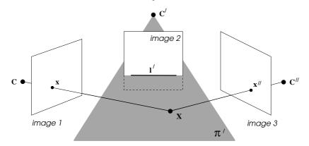
Fig. 15.2. **Point transfer.** A line l' in the second view back-projects to a plane  $\pi'$  in 3-space. A point **x** in the first image defines a ray in 3-space which intersects  $\pi'$  in the point **X**. This point **X** is then imaged as the point  $\mathbf{x}''$  in the third view. Thus, any line l' induces a homography between the first and third views, defined by its back-projected plane  $\pi'$ .
