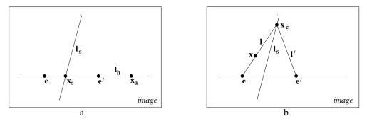
Fig. 9.11. Geometric representation of F for planar motion. (a) The lines  $l_s$  and  $l_h$  constitute the Steiner conic for this motion, which is degenerate. Compare this figure with the conic for general motion shown in figure 9.10. (b) The epipolar line l' corresponding to a point x is constructed as follows: intersect the line defined by the points e and x with the (conic) line  $l_s$ . This intersection point is  $x_c$ . Then l' is the line defined by the points  $x_c$  and e'.
