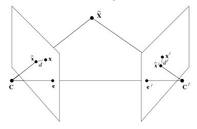
Fig. 12.2. Minimization of geometric error. The estimated 3-space point  $\hat{\mathbf{X}}$  projects to the two images at  $\hat{\mathbf{x}}, \hat{\mathbf{x}}'$ . The corresponding image points  $\hat{\mathbf{x}}, \hat{\mathbf{x}}'$  satisfy the epipolar constraint, unlike the measured points  $\mathbf{x}$  and  $\mathbf{x}'$ . The point  $\hat{\mathbf{X}}$  is chosen so that the reprojection error  $d^2 + d'^2$  is minimized.
