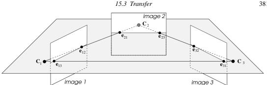
Fig. 15.8. The trifocal plane is defined by the three camera centres. The notation for the epipoles is  $\mathbf{e}_{ij} = \mathsf{P}_i \mathbf{C}_j$ . Epipolar transfer fails for any point **X** on the trifocal plane. If the three camera centres are collinear then there is a one-parameter family of planes containing the three centres.
