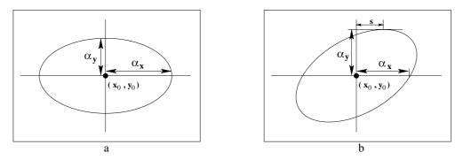
Fig. 8.27. Reading the internal camera parameters K from the calibrating conic. (a) Skew s is zero. (b) Skew s is non-zero. The skew parameter of K (see (6.10-p157), is given by the x-coordinate of the highest point of the conic.
