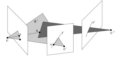
Fig. 15.6. If the plane  $\pi'$  defined by l' is an epipolar plane for the first two views, then any line l'' in the third view gives a point–line–line incidence.
