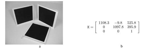
Fig. 8.12. Calibration from metric planes. (a) Three squares provide a simple calibration object. The planes need not be orthogonal. (b) The computed calibration matrix using the algorithm of example 8.18. The image size is  $1024 \times 768$  pixels.
