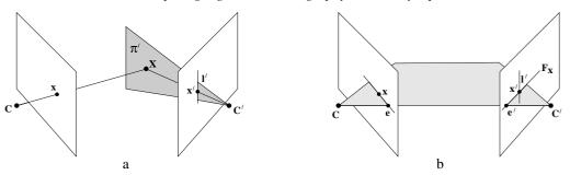
Fig. 13.6. A degenerate homography. (a) The map induced by a plane through the second camera centre is a degenerate homography  $H = [l']_{\times}F$ . The plane  $\pi'$  intersects the second image plane in the line l'. All points in the first view are mapped to points on l' in the second. (b) A point x in the first view is imaged at x', the intersection of l' with the epipolar line Fx of x, so that  $x' = l' \times Fx$ .
