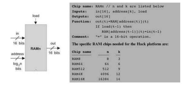
*Read:* To read the contents of register number m, we put m in the address input. The RAM's direct-access logic will select register number m, which will then emit its output value to the RAM's output pin. This is a combinational operation, independent of the clock.
