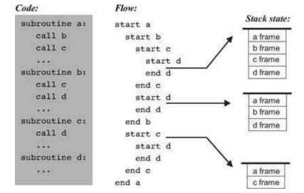
**Figure 8.3** Subroutine calls and stack states associated with three representative points in the program's life cycle. All the layers in the stack are waiting for the current layer to complete its execution, at which point the stack becomes shorter and execution resumes at the level just below the current layer. (Following convention, the stack is drawn as if it grows downward.)
