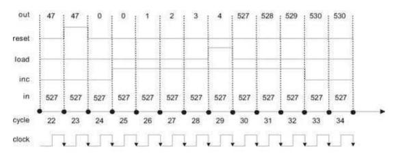
We assume that we start tracking the counter in time unit 22, when its input and output happen to be 527 and 47, respectively. We also assume that the counter's control bits (reset, load, inc) start at 0—all arbitrary assumptions.
