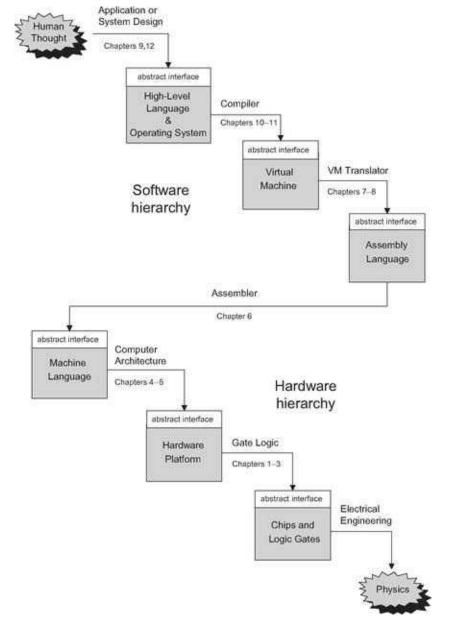
**Figure I.1** The major abstractions underlying the design of a typical computing system. The implementation of each level is accomplished using abstract services and building blocks from the level below.
