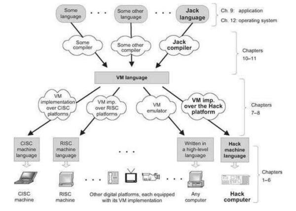
**Figure 7.1** The virtual machine paradigm. Once a high-level program is compiled into VM code, the program can run on any hardware platform equipped with a suitable VM implementation. In this chapter we start building the *VM implementation on the Hack platform* and use a VM emulator like the one depicted on the right.
