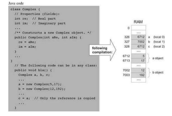
**Figure 11.3** Objects handling. Since memory allocations are run-time dependent, all the shown addresses are arbitrary examples.
