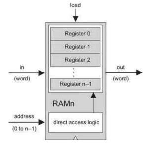
Figure 3.3 RAM chip (conceptual). The width and length of the RAM can vary.
