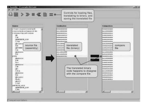
Figure 6.3 Using the supplied assembler to test the code generated by another assembler.
