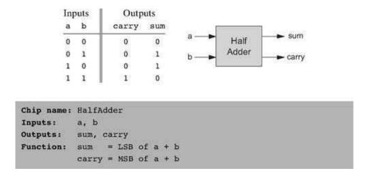
**Figure 2.2** Half-adder, designed to add 2 bits.
