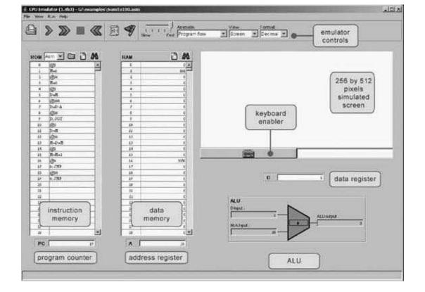
**Figure 4.8** The CPU emulator supplied with the book. The loaded program can be displayed either in symbolic notation (as shown in this screen shot) or in binary code. The screen and the keyboard are not used by this particular program.
