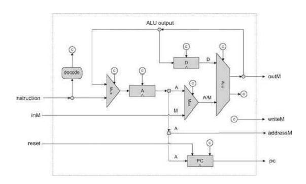
**Figure 5.9** Proposed CPU implementation. The diagram shows only *data* and *address paths*, namely, wires that carry data and addresses from one place to another. The diagram does not show the CPU's *control logic*, except for inputs and outputs of control bits, labeled with a circled "c". Thus it should be viewed as an incomplete chip diagram.
