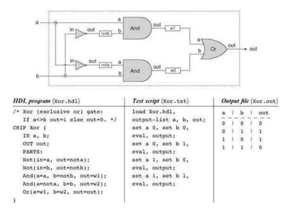
Figure 1.6 HDL implementation of a Xor gate.
