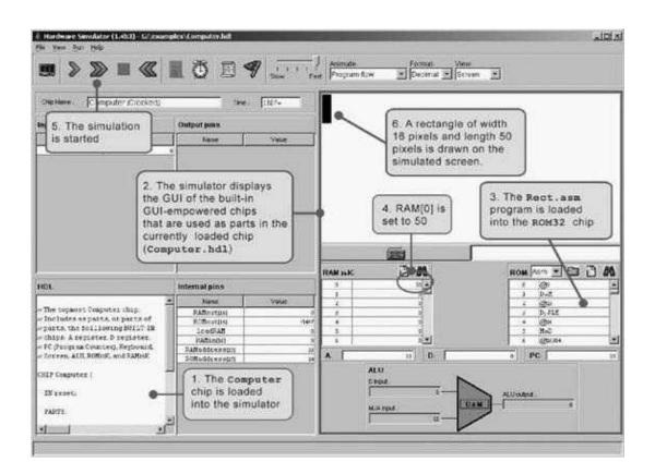
**Figure 5.11** Testing the Computer chip on the hardware simulator. The Rect program draws a rectangle of width 16 pixels and length RAM[0] at the top left of the screen. Note that the program is correct. Thus, if it does not work properly, it means that the computer platform on which it runs (Computer.hdl and/or some of its lower-level parts) is buggy.
