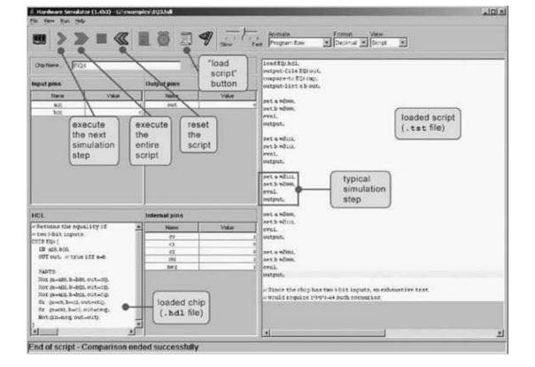
**Figure B.2** Typical hardware simulation session, shown at the script's end. The loaded script is identical to EQ3.tst from figure B.1, except that some white space was added to improve readability.
